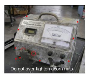
Reassemble the case. Make sure the fan wires fall to the bottom of the case and are clear of the carbon pile as you lower the top to the bottom. Replace all screws. Make the acorn nuts snug. DO NOT TIGHTEN.
