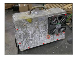
Begin by removing all sheet metal screws • Loosen, but do not remove acorn nuts 🔾
