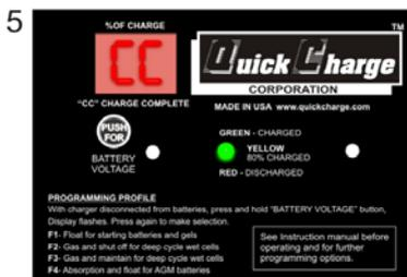
Shortly after the cycle reaches 99%, the cycle terminates and displays CC "Charge Complete". The LED will be solid green if the charger shuts off, or it will flicker, if set to maintain. The flickering is the charger regulating on and off.
