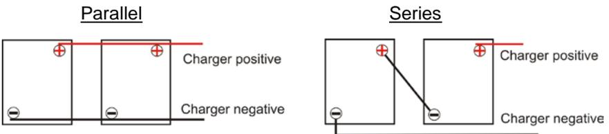
When batteries are connected in Parallel the battery amp hour capacity is additive and the voltage remains the same.
