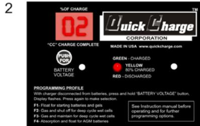
After displaying the profile for a few seconds, the LED will turn solid red, and display 02 on a discharged battery. The time it spends there depends on how deeply discharged it is, it may be hours before it starts to move higher.
