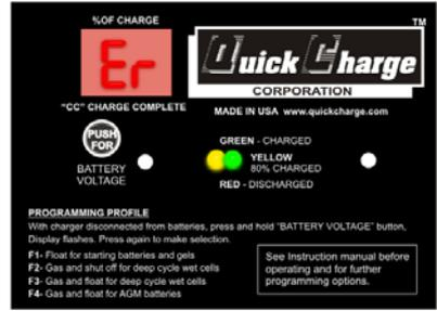
Error is displayed at the end of a cycle and a green/yellow alternating LED if a minimum voltage is not reached in the time given. See trouble shooting for more info.
