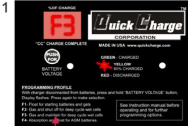
Connect red lead to battery positive, black to negative. Plug charger into AC power. The charger will display the profile it is set to, and the LED will flash red. By the descriptions, verify it matches your battery type. If not, disconnect a battery lead, and go to programming section.
